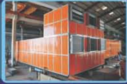
Air Handling Units
