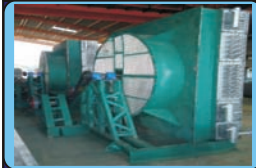
CNG Air Exchangers
