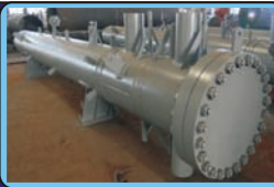
HP / LP Feed Water Heaters
