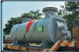
Compressor Inter Coolers
